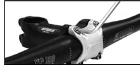
Place handlebar into stem and replace front plate making sure the handlebar is equal in length on both sides.
