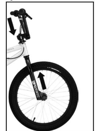
Once desired handlebar position is found you will now need to tighten the bolts on the front plate of the stem.
